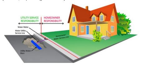
Most meters are housed in outdoor meter boxes near the edge of your property. The county is responsible for maintaining the portion of the service line that runs from the water main in the street up to and including the water meter. From the meter to your home's internal plumbing, however, the **property owner is responsible** for maintaining that section of the service line.
